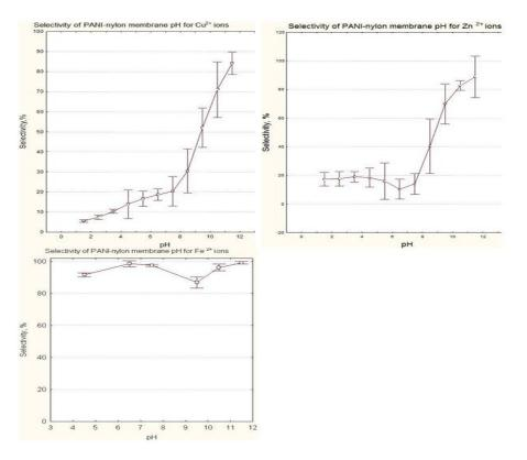
Figure 2: Dependence of the selectivity of the membrane nylon-PANI from the pH of a solution for metal ions: Fe<sup>2+</sup>, Cu<sup>2+</sup>, Zn<sup>2+</sup>.
