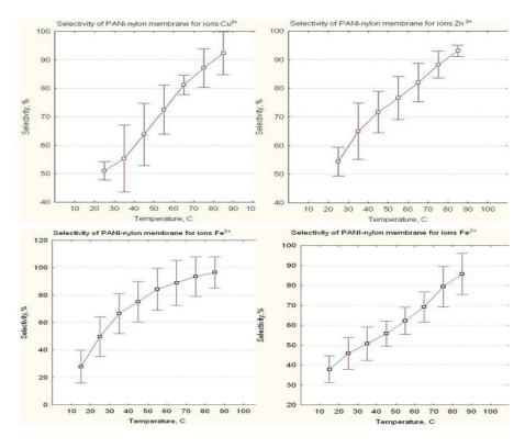
Figure 1: The dependence of selectivity of the membrane nylon-PANI from the solution temperature for metal ions: Fe<sup>3+</sup>, Fe<sup>2+</sup>, Cu<sup>2+</sup>, Zn<sup>2+</sup>.
